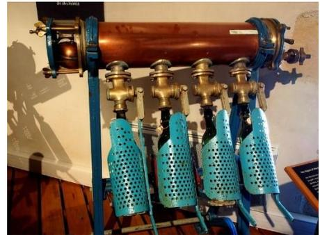
Figure 58. Even older models had a mechanical shut off valve that would prevent the bottles from overfilling if the regular valve failed. By AlfvánBeem (Own work) [CC0], via Wikimedia Commons.
